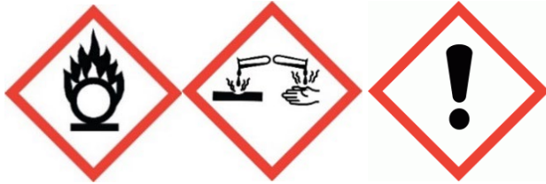
Flame over circle Corrosion Exclamation mark
